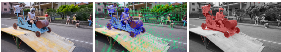
Figure 1: Example frame from our results. Left: input frame. Center: tracked features are color-coded by model fit (inliers are green, outliers are blue) with lines showing the difference to the background model’s prediction. Right: dense segmentation.
