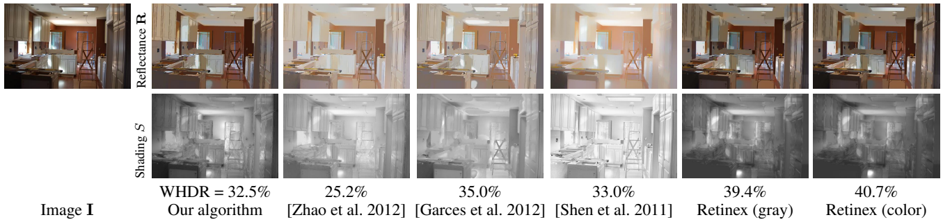
Figure 86: Visual comparison of our algorithm against several recent open-source algorithms. Each algorithm uses the best parameters found from training (i.e., minimizes mean WHDR 10% across all photos). OpenSurfaces Photo ID: 69088.
