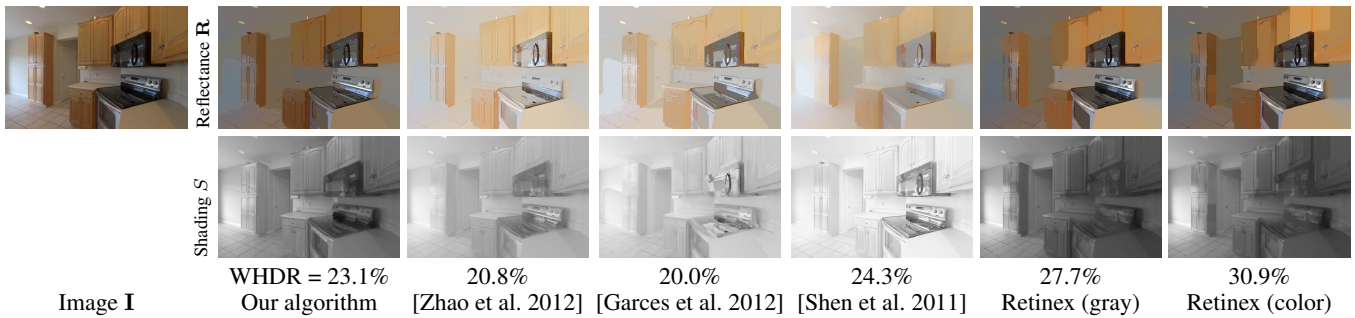
Figure 40: Visual comparison of our algorithm against several recent open-source algorithms. Each algorithm uses the best parameters found from training (i.e., minimizes mean WHDR 10% across all photos). OpenSurfaces Photo ID: 118512.
