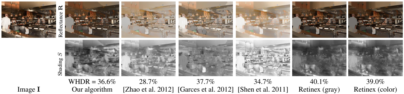
Figure 54: Visual comparison of our algorithm against several recent open-source algorithms. Each algorithm uses the best parameters found from training (i.e., minimizes mean WHDR 10% across all photos). OpenSurfaces Photo ID: 60889.
