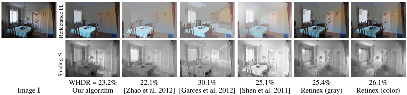
Figure 91: Visual comparison of our algorithm against several recent open-source algorithms. Each algorithm uses the best parameters found from training (i.e., minimizes mean WHDR_{10\%} across all photos). OpenSurfaces Photo ID: 11902.
