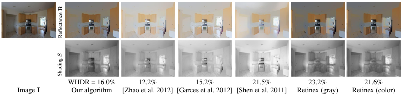
Figure 51: Visual comparison of our algorithm against several recent open-source algorithms. Each algorithm uses the best parameters found from training (i.e., minimizes mean WHDR 10% across all photos). OpenSurfaces Photo ID: 118510.
