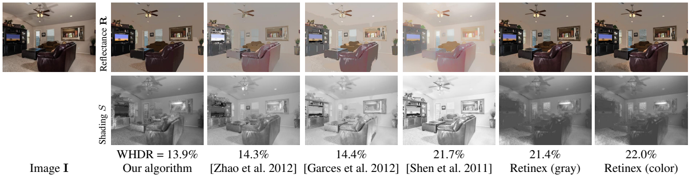
Figure 88: Visual comparison of our algorithm against several recent open-source algorithms. Each algorithm uses the best parameters found from training (i.e., minimizes mean WHDR 10% across all photos). OpenSurfaces Photo ID: 59157.
