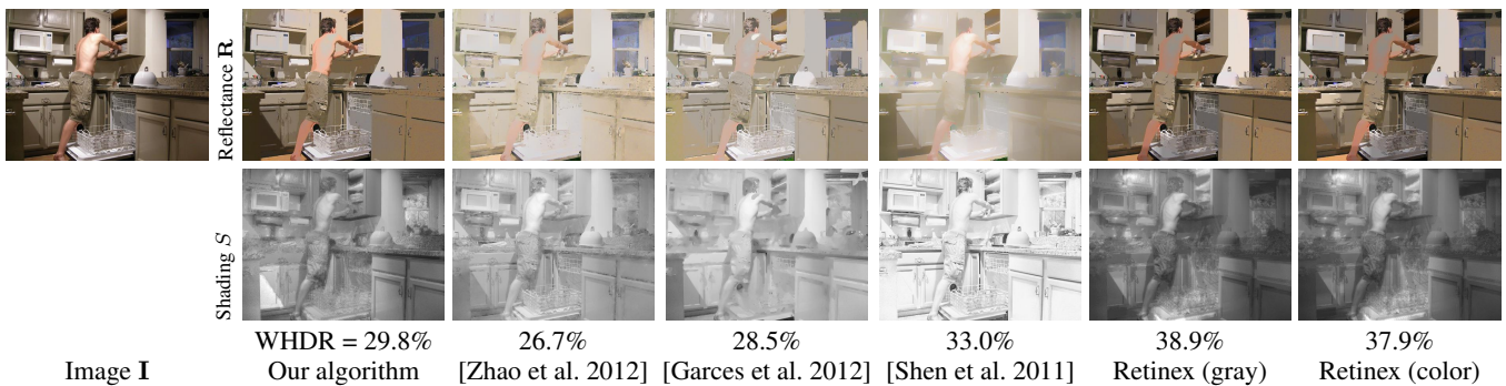
Figure 70: Visual comparison of our algorithm against several recent open-source algorithms. Each algorithm uses the best parameters found from training (i.e., minimizes mean WHDR_{10\%} across all photos). OpenSurfaces Photo ID: 69278.
