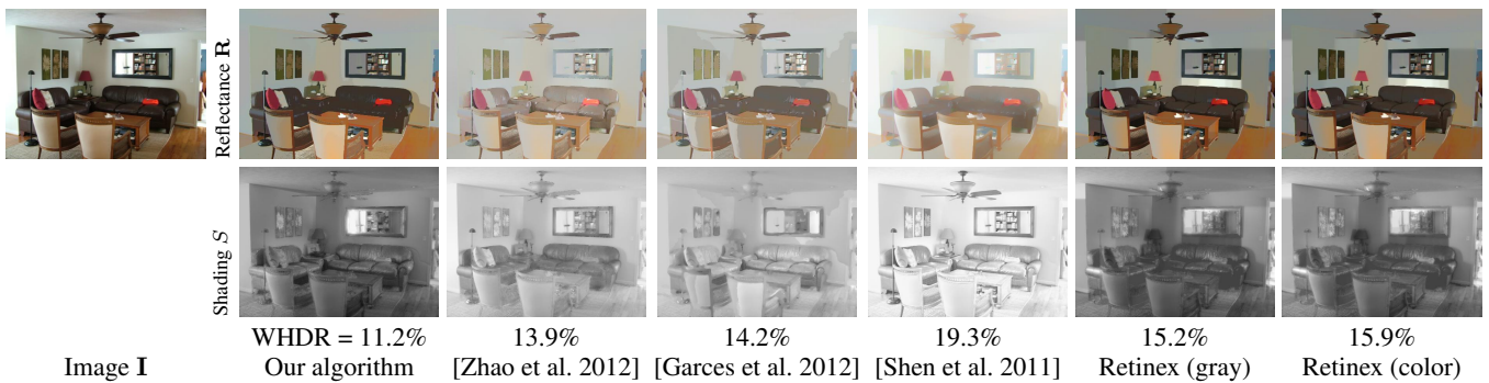
Figure 45: Visual comparison of our algorithm against several recent open-source algorithms. Each algorithm uses the best parameters found from training (i.e., minimizes mean WHDR_{10\%} across all photos). OpenSurfaces Photo ID: 34942.
