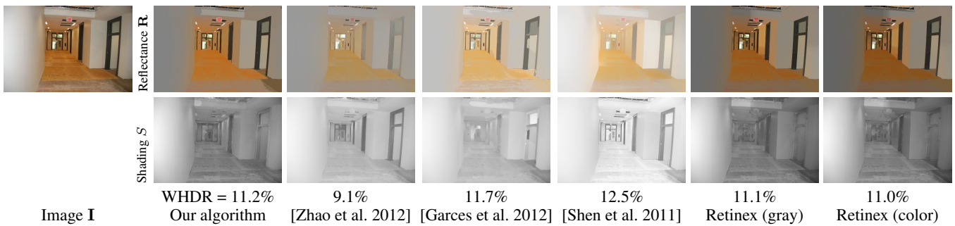
Figure 61: Visual comparison of our algorithm against several recent open-source algorithms. Each algorithm uses the best parameters found from training (i.e., minimizes mean WHDR 10% across all photos). OpenSurfaces Photo ID: 108975.
