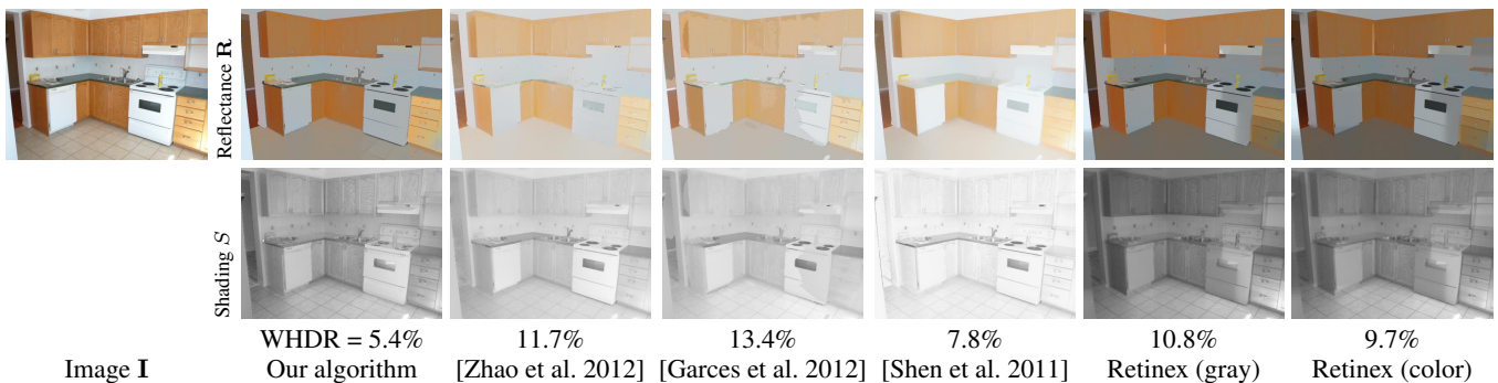
Figure 85: Visual comparison of our algorithm against several recent open-source algorithms. Each algorithm uses the best parameters found from training (i.e., minimizes mean WHDR 10% across all photos). OpenSurfaces Photo ID: 66411.
