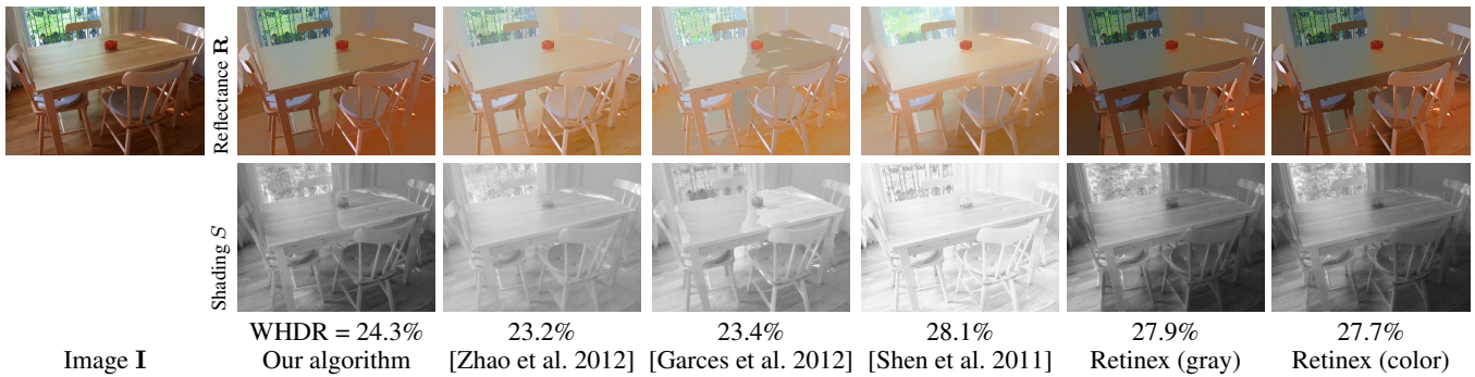
Figure 60: Visual comparison of our algorithm against several recent open-source algorithms. Each algorithm uses the best parameters found from training (i.e., minimizes mean WHDR 10% across all photos). OpenSurfaces Photo ID: 89875.
