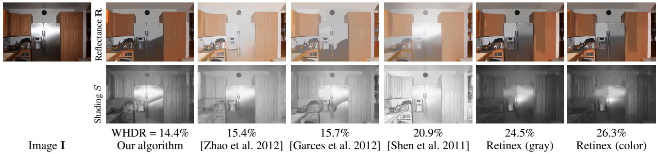
Figure 62: Visual comparison of our algorithm against several recent open-source algorithms. Each algorithm uses the best parameters found from training (i.e., minimizes mean WHDR 10% across all photos). OpenSurfaces Photo ID: 3446.
