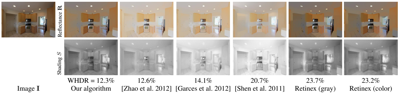
Figure 52: Visual comparison of our algorithm against several recent open-source algorithms. Each algorithm uses the best parameters found from training (i.e., minimizes mean WHDR 10% across all photos). OpenSurfaces Photo ID: 118509.
