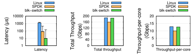
Figure 12: blk-switch is able to maintain low average and tail latencies even when applications operate at throughput close to 200Gbps. The experiment uses 16 L-apps and 16 T-apps running across 16 cores from two NUMA nodes.
