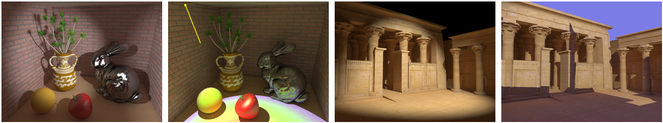
Figure 1: Two scenes rendered under different lighting configurations, relit at 10-20 fps with multiple bounces of indirect illumination. These scenes include up to 2.1 million polygons, diffuse and glossy materials and procedural light shaders.
