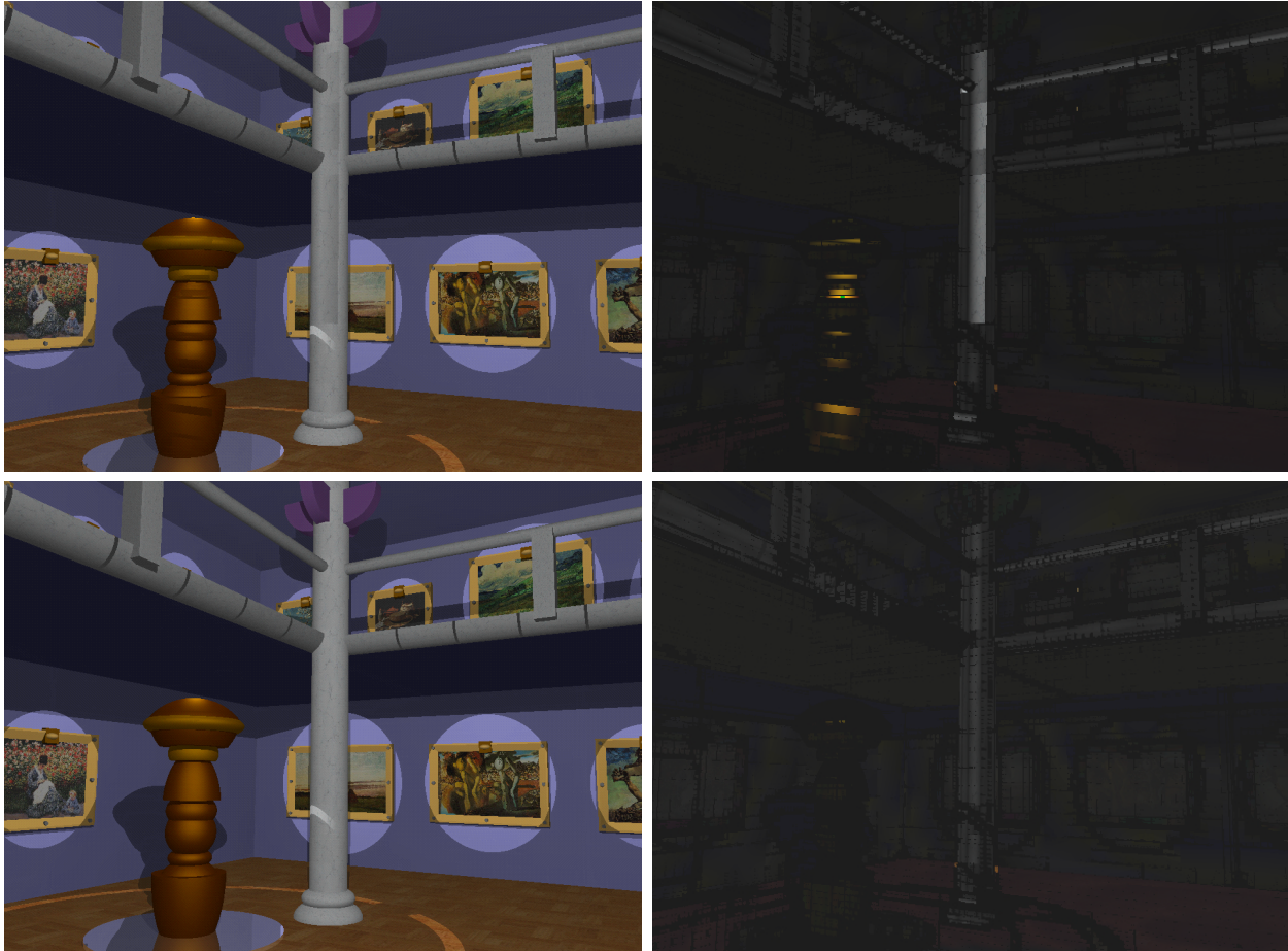
Figure 4-27: Error refinement for the museum scene. Top row: without non-linearity detection. Bottom row: with non-linearity detection and \epsilon = 0.5 . Right column: scaled difference images.
