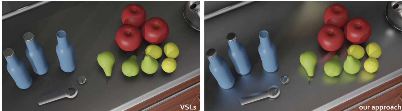
Figure 1: Comparison of our approach with Virtual Spherical Lights (VSLs). Left: VSLs fail to capture small local glossy reflections (time: 6 m 26 s). Right: our method (time: 4 m 59 s) computes these reflections more efficiently and accurately by using visibility approximations for the low-rank global light transport, and local lights for the high-rank localized light transport.
