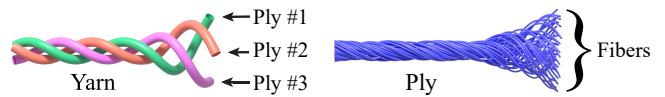
Figure 3: Fabric structure: a yarn normally consists of multiple sub-stands called plies. Each ply in turn contains tens to hundreds of micron-diameter fibers.
