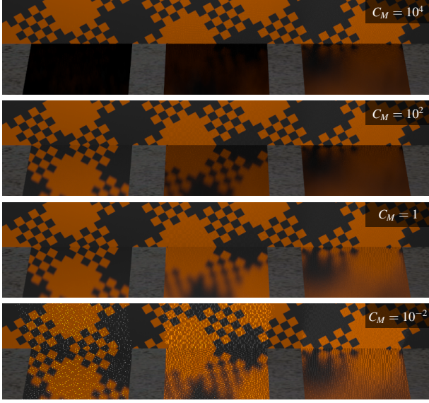
Figure 5: The effect of different values of our C_M parameter. This scene contains three surfaces with decreasing gloss sharpness from left to right. Setting C_M too high (e.g., top) excludes energy even from sharp reflections, while setting it too low (e.g., bottom) results in objectionable noise from caustics and other problematic paths. Our results use the somewhat conservative value of C_M = 10^2 .
