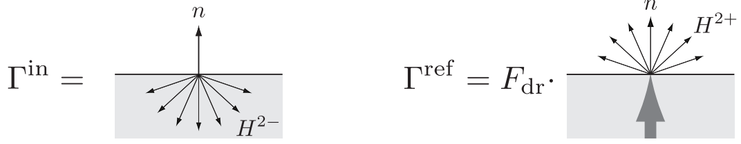
Figure 6: The Robin boundary conditions (38) specify that the net inward flux \Gamma^{\text{in}} matches the overall portion F_{\text{dr}} of the outward flux that is reflected by interface effects (this is denoted by \Gamma^{\text{ref}} ).
