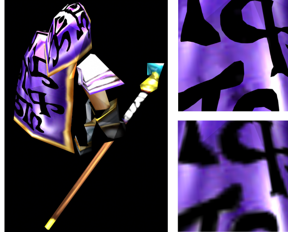
Figure 11: Comparisons of wizard model. Left: Antialiased rendering of model using an FBT skin. Right: zoomed-in comparison (Top: FBT; Bottom: original raster skin). Artwork from Warcraft III®: Reign of Chaos™ provided courtesy of Blizzard Entertainment.
