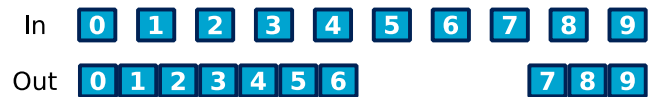
Figure 1: Illustration of the perturbation of the time distribution of packets between homogeneous input to, and compressed output from, a wide-area network.
