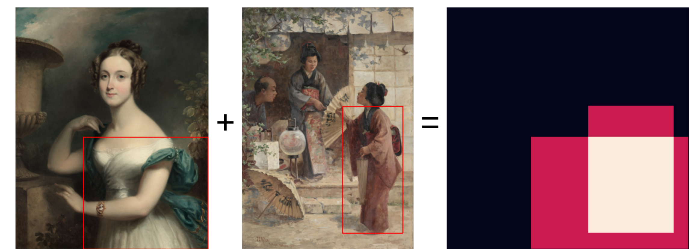
Two bounding boxes for fabrics are combined into a material heatmap. Overlapping regions becomes brighter. With hundreds of bounding boxes, the color gradients become smooth, with the brighter areas marking the spatial location where materials are more likely to be depicted.
