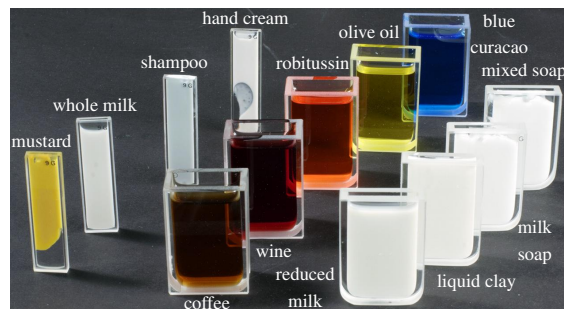
Figure 7: Measured materials in glass cells of width w = 1, 10 , and 2.5 mm, from left to right. It is not necessary for all of the cell to be filled, as long as there exists a homogeneous region of size comparable to the beam diameter (e.g., hand cream).
