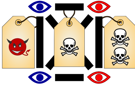
Figure 4.10: Failure Disagreement Observer Graph Observers are shown as eyes, with darker blue observers on the left, and lighter, outlined red observers on the right. Note that the edges between each pair of observers are labeled with the set of failures they want to tolerate. Crash (safe, but not live) failures are denoted with a skull, and byzantine failures with a devil. All edges except the rightmost and leftmost share a central label.
